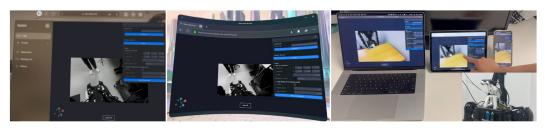
Figure 12: **Our web-based cross-platform system enables access across different devices.** Left: Apple Vision Pro. Middle: Meta Quest. Right: Macbook, iPad and iPhone. On VR devices, the users can enter an immersive session to start teleoperation with hand and wrist pose streaming. On other devices, hand and wrist streaming are not available but the user can still see the streamed images and control the robot's active neck by dragging on the devices' screen.
