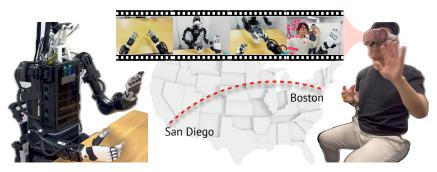
Figure 9: **Our system enables cross-country teleoperation over the internet.** The operator at Boston, USA can operate a robot at San Diego, USA (approximately 3000 miles away). The robot and operator pictures are flipped left to right for better illustration.
