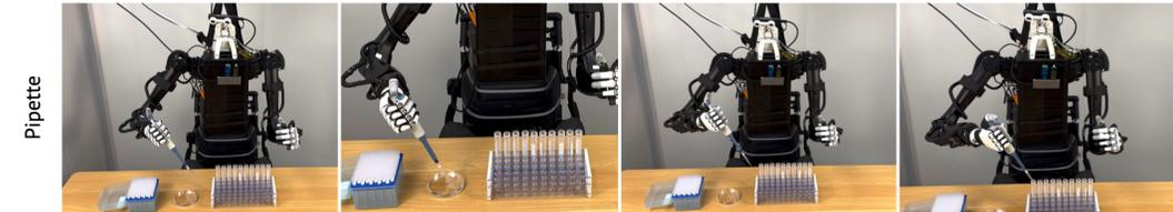
(c) The robot utilizes its thumb DoF to control a pipette to transfer liquid from a petri dish to a centrifuge tube. The diameter of the tube is only  $1.5\text{cm}$  so it requires high precision to complete the task.
