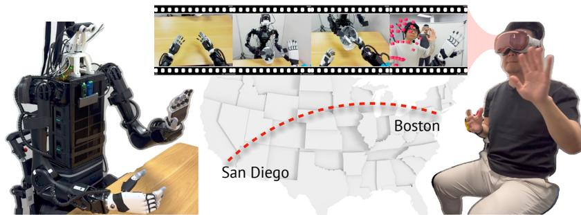
Figure 9: **Our system enables cross-country teleoperation over the internet.** The operator at Boston, USA can operate a robot at San Diego, USA (approximately 3000 miles away). The robot and operator pictures are flipped left to right for better illustration.
